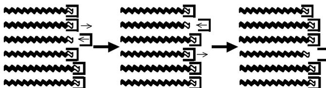
**Figure 1.4:** Illustrating a capping and uncapping style mechanism where each chain may briefly uncap itself, propagate and then re-cap itself. In this mechanism, the dormant to active reaction is unimolecular.
