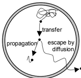
**Figure 1.7:** A schematic representation of the standard model for the exit of a monomeric radical from a latex particle. Once a chain-transfer to monomer event occurs, the monomeric radical can then either add to monomer (starting a new chain) or escape from the particle by diffusion. The passage through the interface is not rate-determining.
