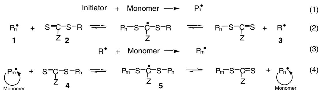
**Scheme 1.1:** The RAFT mechanism proposed by Rizzardo *et al.*<sup>1,4,34,35</sup> The crucial reaction for providing living character to the system is the equilibrium shown in reaction 4.
