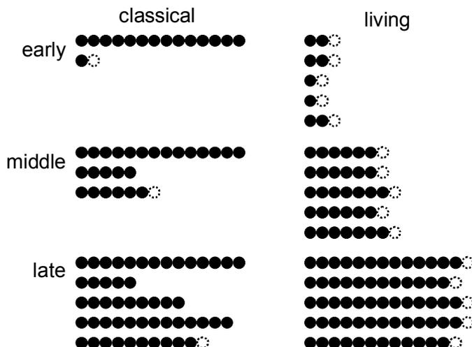
**Figure 1.1:** A comparison of classical and living polymerizations illustrating the chain length and number of growing centers (shown with dotted ends) at three stages during the reaction.
