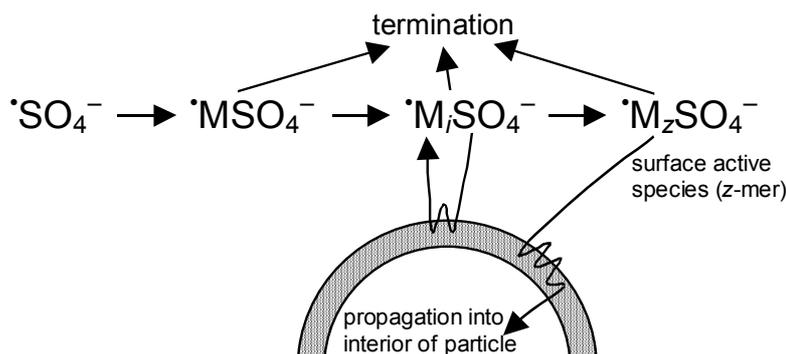
**Figure 1.6:** A schematic representation of the Maxwell–Morrison model<sup>54,55</sup> for the entry of oligomeric radicals into latex particles. In this model, the entering species is an initiator-derived oligomeric radical (a *z*-mer) that is surface-active; oligomers that are shorter than a *z*-mer tend to be too water soluble to enter due to the charged initiator fragment. The passage through the interface is not rate-determining.
