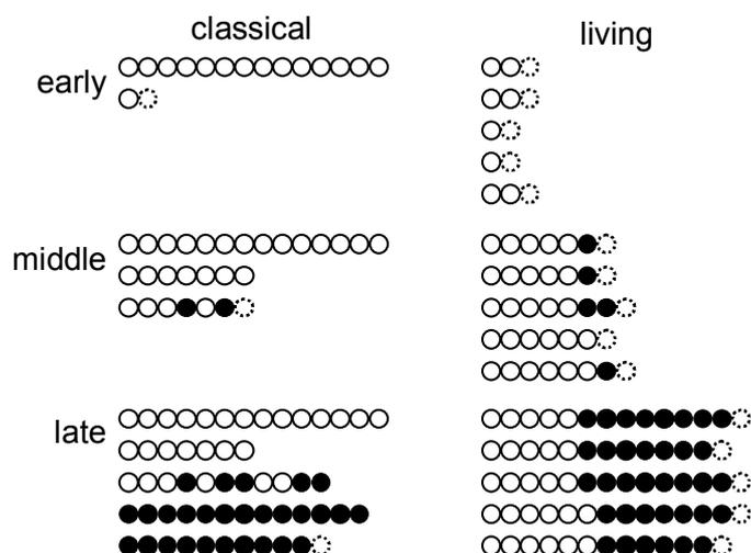
**Figure 1.2:** Illustration of how block copolymers are easily made with living polymerizations, but the same reaction would produce a heterogeneous mix of copolymers with a classical polymerization. Closed circles represent one monomer, open circles a second monomer and dotted ends growing centers. Three stages during the reaction are shown.
