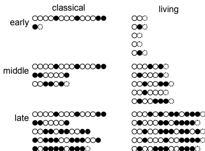
**Figure 1.3:** Illustrating how gradient copolymers are easily made with living polymerizations, but the same reaction would produce a heterogeneous mix of copolymers with a classical polymerization. Symbols as per Fig. 1.2.
