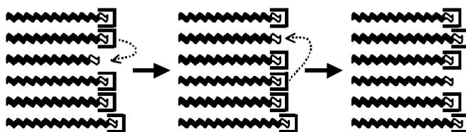
**Figure 1.5:** Illustrating a cap-swapping mechanism where the dormant species exchange their end-cap for the ability to grow. In the RAFT mechanism, the dithiocarbonyl functional group is the end-cap that is exchanged for radical activity. Here, the dormant to active reaction is bimolecular.
